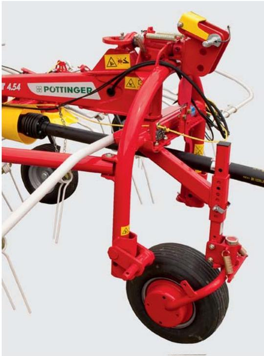
**Ground tracking and forage protection are the key objectives of HIT rotary tedders. An optional jockey wheel on the pivoting headstock tracks the ground immediately in front of the tine path and responds to each undulation. The result: Clean forage, lower raw ash content and improved livestock health.**
