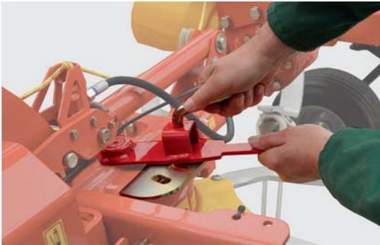
**Actively setting the wheels at an angle causes the tedder to run diagonally so the forage is directed onto the mown area. Neighbouring crops remain untouched. Because the wheels can be set to the left or right, fenceline tedding can be activated in any driving direction.**
