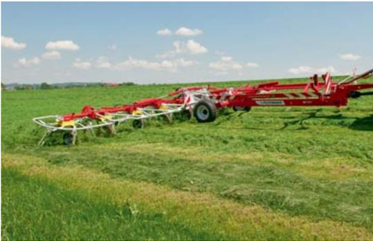
**The trailed HIT T tedders with 10 or 12 rotors are designed for high output tedding. To meet the requirement of wider working widths and still provide the best possible ground tracking, the rotor units are linked together by individual hinge points. Combined with the chassis wheels guiding the rotors, HIT T tedders guarantee a perfect operation even at higher working speeds.**
